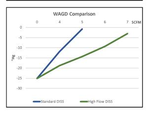
The graphs above represent the difference in pressure drop as flow of gas or vacuum increases.
